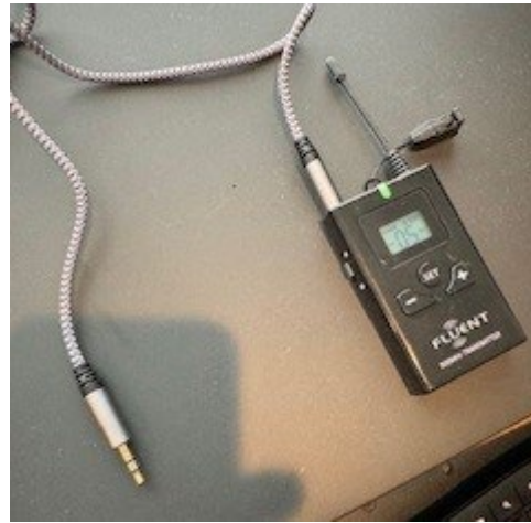
Figure 4 Transmitter connected to audio cable
