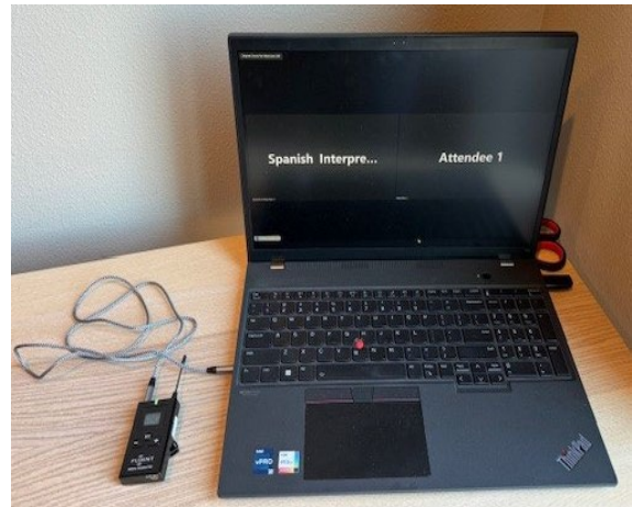
Figure 6 Laptop connected to transmitter programmed to Language 1 channel.
